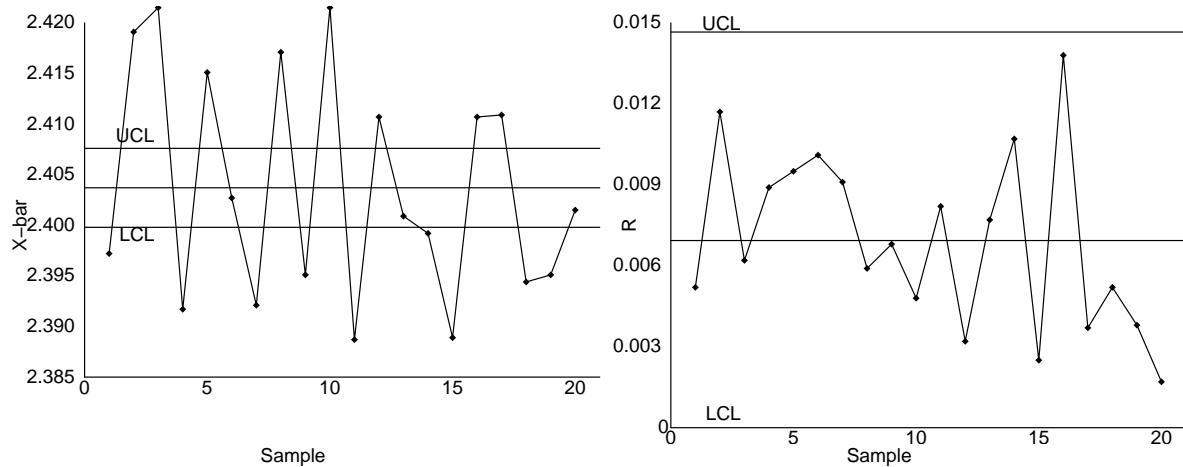
Although none of the points in  $R$ -chart is outside of the limits, there are many values fall outside control limits in the  $\bar{X}$ -chart.
