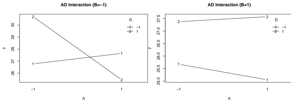
It can be argued that when  $B = 1$  that there is essentially no interaction between  $A$  and  $D$ . Clearly when  $B = -1$ , the presence of a high level of  $D$  produces a strong negative effect of Factor  $A$  on the response.
