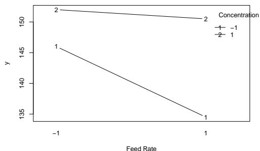
The mean viscosity does not change much at high level of concentration, while it changes a lot at low concentration.
