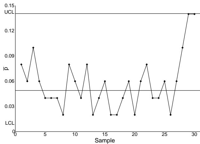
Although there are a few points closed to the upper limit, the process appears to be in control as well.
